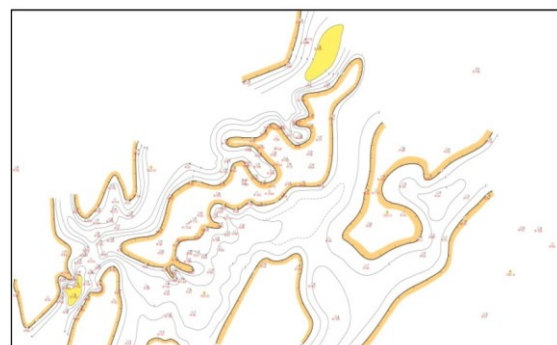
Figure 16: Sand Isolith Map of Unit-I, TS-IV showing channel features and channel direction
