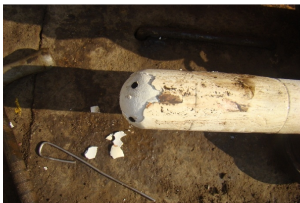
Figure 5: Well-B: Scale came out along with CTU
