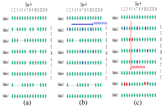
Fig.5: Offset volume showing missing traces (a), interpolation along inline direction (b) and interpolation along xline direction (c)
