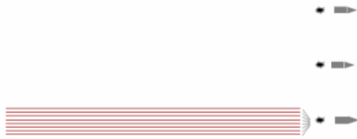
Figure 3: A wide-azimuth configuration using one streamer vessel and two source vessels; each vessel has a single-source array.
