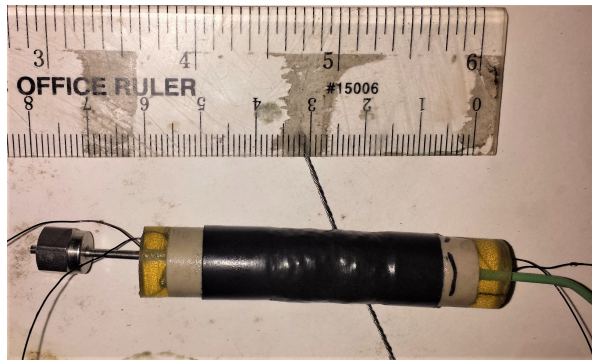
Figure 3: Sample of coarse-grained quartz sand between 2 ultrasonic transducers, covered with a heat-shrink sleeve, length: 21 mm, diameter: 12.6 mm
