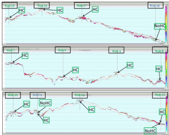
Fig.9. Arbitrary lines (3 nos.) showing the coloured impressions or regions of hydrocarbon (9) and non-hydrocarbon (3) wells.
