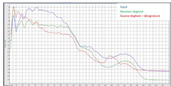
Figure 5 (d): Stack amplitude spectra; receiver & source-side de-ghosting and 1-d de-signature.
