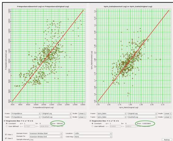
Figure 11. Cross-plot of Inverted log vs Original log of P-impedance (left) and Vp/Vs ratio (right)
