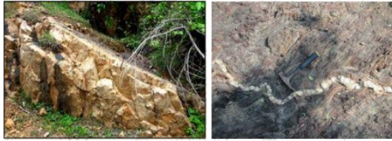
Figure 9.1 Exposure of fractured and jointed quartzite, Rathamgutta hill, Manuguru (Left) and Exposure of phyllite with floded silicate vains rocks near Bugga Dolomitic limestone exposed near SCCL, Manuguru Coal Mines (Right)
