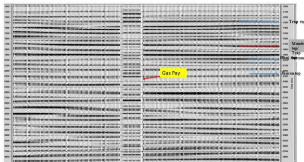
Figure-8(b): The well tie of VSP corridor stack (of W-4 well) spliced at well location on the (PP + PSSP) mixed mode depth section scaled to time of line LO-2 also confirms the genuine mapping of energy on mixed mode section and proper calibration.
