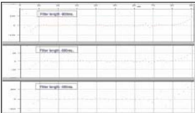
Fig.7: Shows the results of the Filter testing – Filters designed with different filter lengths applied on the extracted wavelet.
