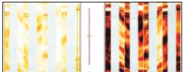
Fig. 7: Static and Dynamic Images of the interval encompassing Zones 30 to 33. High angle erosional cut - fill. Well likely to be located not far from cut-edge.
