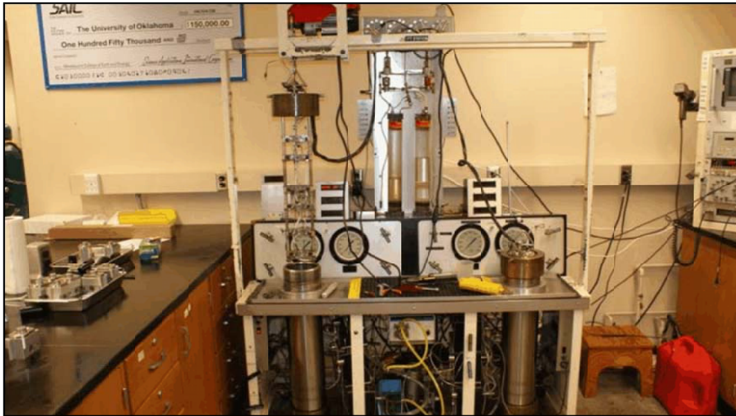
Fig. 6 Picture showing the apparatus used for Pulse-Transmission method (OU-IC 3 lab).
