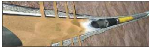
Fig. 9: Schematic representation of a Plug and Perforate (PNP) completion.
