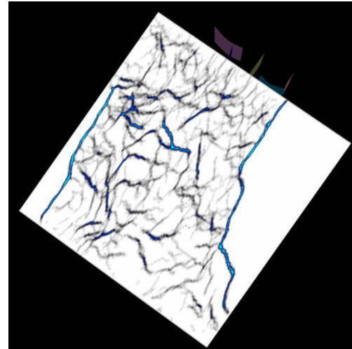
Fig:7 Ant Tracked Volume showing sub seismic lineaments
